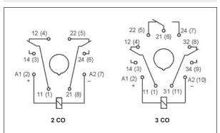
Note: the indicated polarization of the supply refers to the relays with extra equipment  $\boldsymbol{\mathsf{D}}$  - surge suppression element (diode) - for DC coils only.
