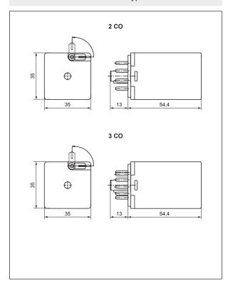
**Dimensions** - plug-in version, with test button (no latching) or with plug (no manual operation)
