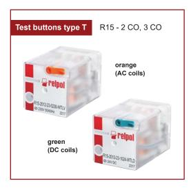
**Test buttons (no latching)** are recommended for R2N...WT, R3N...WT, R4N...WT, R15...WT 2 CO, R15...WT 3 CO relays - **for applications that do not allow permanent contact latching**. By manual operation (pressing the button) relay contacts can get switched for as long time as long the button is pressed. Contacts return to initial position as soon as pressure is released from the button. Those operations can be done while the coil is deenergized **§**.
