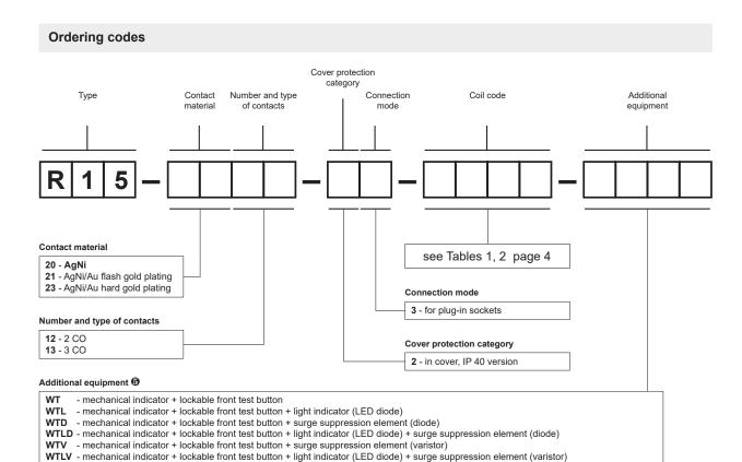
**ூ** T - orange colour (AC coils), green (DC coils). **WT** - standard equipment of relays for plug-in sockets. **WTD, WTLD** - available only in relays with DC coils. **WTV, WTLV** - only with AC coils.
