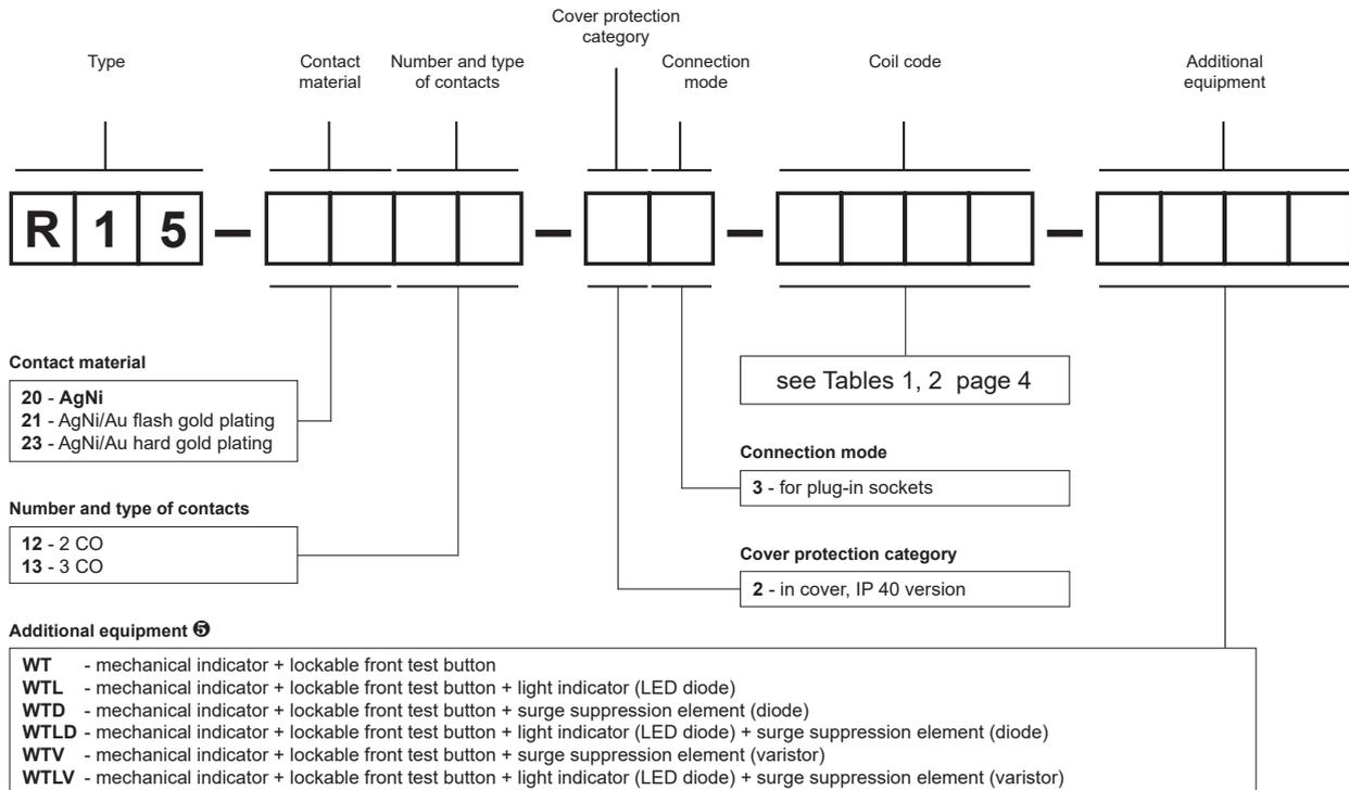
⑤ T - orange colour (AC coils), green (DC coils). WT - standard equipment of relays for plug-in sockets. WTD, WTLD - available only in relays with DC coils. WTV, WTLV - only with AC coils.
