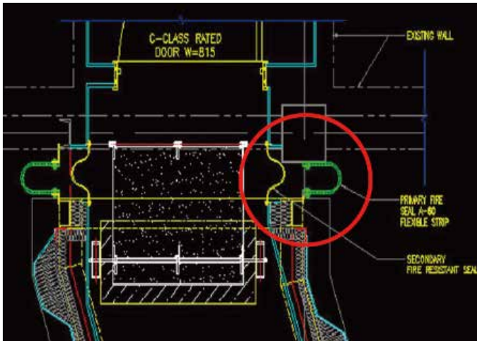
BARZAN Offshore Project of HHI [access corridor flexible seal]
