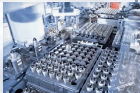
Assembly and testing of pressure switches on semi or fully automated plants.
