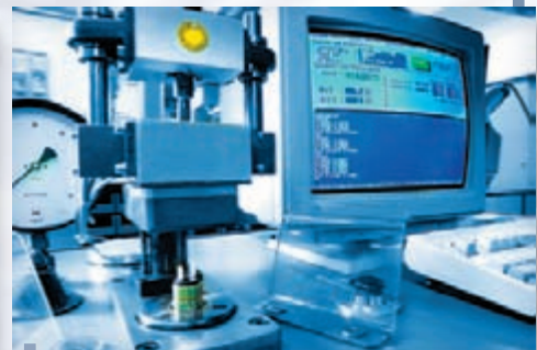
Fully-automatic setting of switching point with computer-aided documentation of results.
